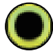
Default point icon (chart plotter, radar and weather displays (black circle in yellow circle)
