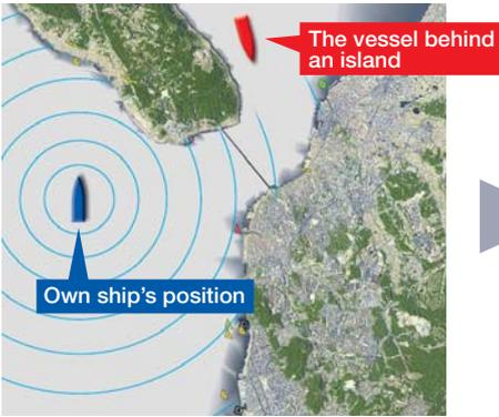
AIS targets can show that a vessel is coming from behind an island, where a Radar beam does not reach.
