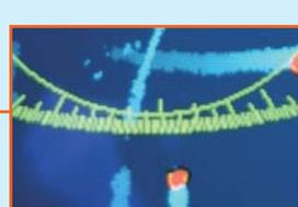
Clearance between markings of the bearing scale is changed according to the proximity between own ship and the bearing circle, as shown in the images on the left-hand side. It helps to grasp the bearing to the target echo without using EBL.
